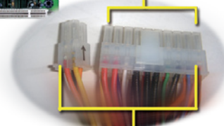
20+4 pin-ATX power connector
