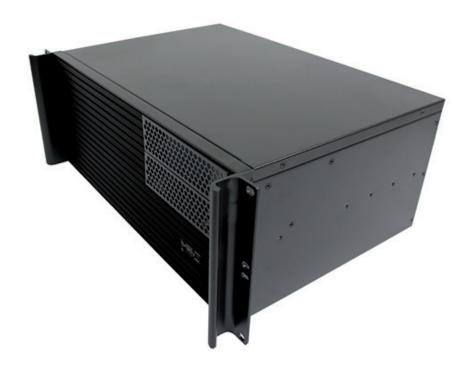
The Hatteland Technology Short Rack is a 19" 4U short rack computer that can be mounted in shallow racks (300 mm). The series is developed and designed by Hatteland Technology and is built with industry-class components for safe operation for a long time in demanding environments. The HT Short Rack series has a variety of processor, hard disk and memory options.
