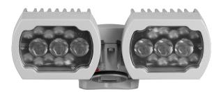
The illuminator accessory has a dual-pod housing incorporating a combination of long-life IR (850 nm/940 nm) + White light LEDs. The illuminator enables viewing of objects even in total darkness, ensuring high-quality images regardless of the lighting conditions.
