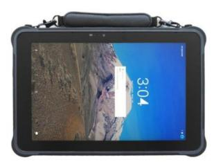
ST935K is a powerful rugged industrial tablet. This device has great battery performance and a screen with 1920x1200 full HD resolution, along with 450 NITS brightness for good readability even in direct sunlight. It is running on an Intel Atom Z8350 1,44GHz Quad-core CPU and is IP65 Rated for harsh environments. Because of this, ST935K can be deployed in many different areas such as manufacturing, logistics, warehouse/asset/animal management, and much more.
